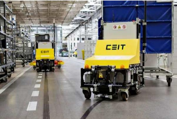
**Fig. 13** Automated tugger guided by a magnetic tape [18]
