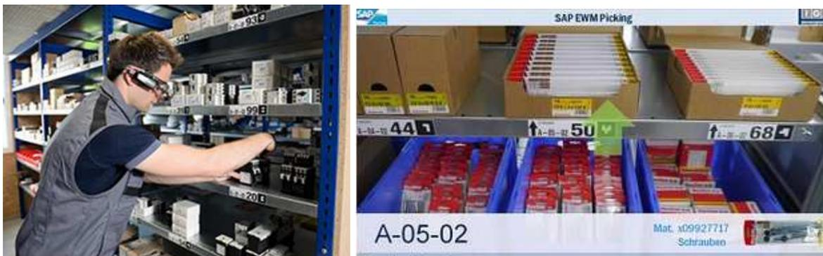
**Fig. 11** Picking by means of smartglasses [3]
