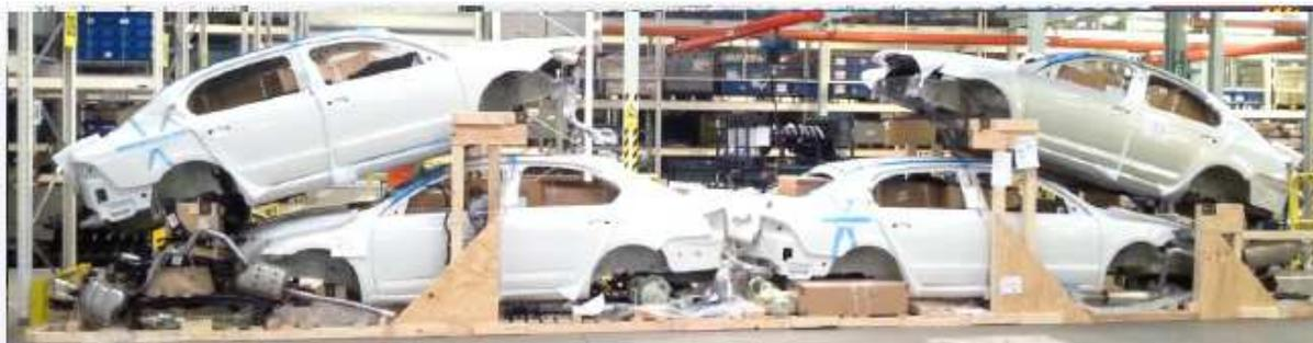
**Fig. 21** Wooden transport frame for car bodies [18]
