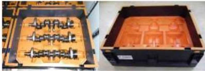
**Fig. 18** Special packaging for components of a single type [18]
