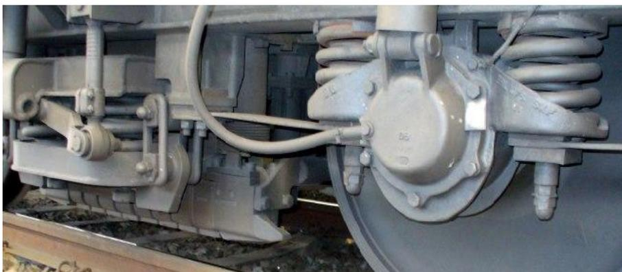
Fig. 10 Electromagnetic rail brake
