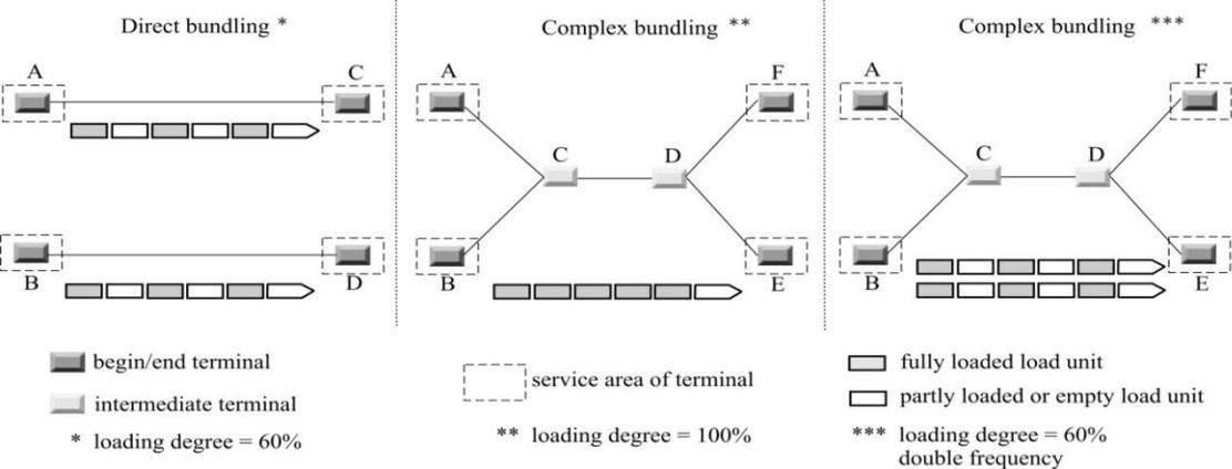
Fig. 1 Principle of the direct and complex bundling
